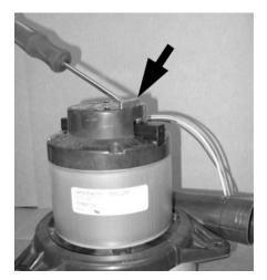
**2.** Replace carbon brush (A), by disconnecting at the terminal connection (B).
